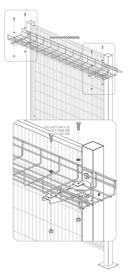
**Frontal Steel Cable Trunking** ASSEMBLY INSTRUCTION - FOR SINGLE UPPER GUIDE SLIDING DOOR
