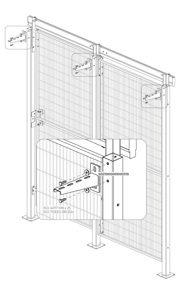
**Frontal Steel Cable Trunking** ASSEMBLY INSTRUCTION - FOR SINGLE UPPER GUIDE SLIDING DOOR
